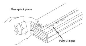
Figure 8. Turning the printer ON
